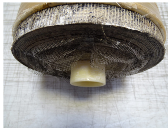
Figure 5.1: Telescopic effect in a spiral-wound module.
